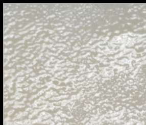
Competitor bonding layer Non-homogeneous, jagged surface
